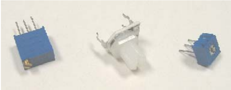
Figure 5-2 A Few Potentiometer Examples
