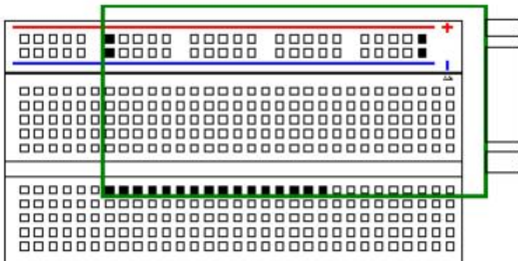
Figure 2: Mounting Stamp the Stack on a Breadboard
