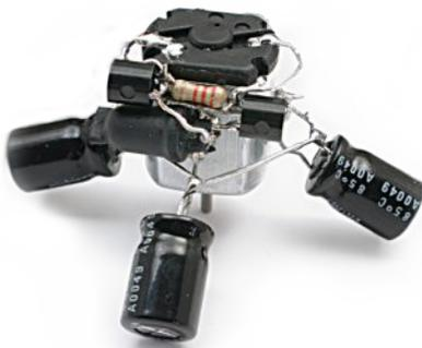
4) Skip ahead, and build your solarengine circuit. When done, install it tight to one side of the motor. The right leg of the 3904 goes to the other motor connection tab, the 3904 left leg solders to the motor body ('-'), and the left leg of the 3906 solders to any point of the '+' ring.
