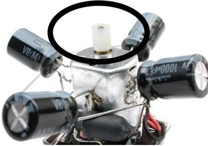
7) If your silicone tubing is a bit long, make sure you cut it down so it's no longer than the length of the motor shaft.
