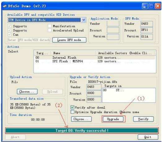
5. Shut down and reactivate power to use new firmware.
