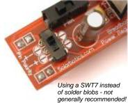
Power your BVRv2 with any DC power source rated 6~18 volts (35VDC max!). The power regulator will warm when powered with over 12V (that's ok).
