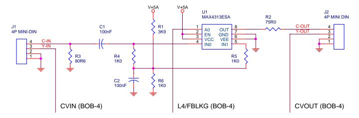
Low-impedance power supply bypass capacitors must be added. 4.7~22uF tantalum in parallel with 100~220nF ceramic is suggested. Bypasses must connect to MAX4313 power and ground pins with minimum length. Due to analog signal processing delays in the luma channel in BOB-4 (~100nS), FBLKG slightly leads luma output. This chroma channel processor circuit helps equalize the delay differential, but closer scrutiny might be necessary in critical applications.
