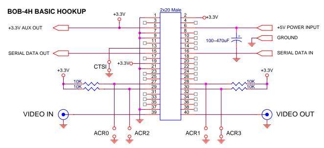
Note: +3.3V connection bubbles must be linked together.
