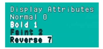
In 2bpp (two bits per pixel) fonts, a pixel can be 00, 01 or 10. Halftone pixels are rendered gray in local video mode. See table and illustration below:
