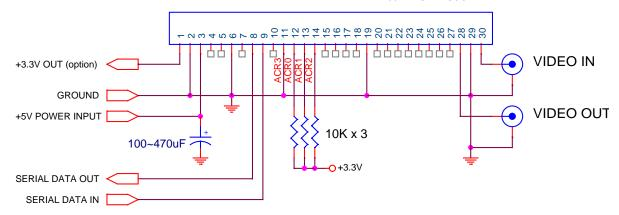
BOB-4S (30-pin SIMM version) does not output 3.3V power on pin 1 by default. See **Pin Description Table**. Pins 1~3 are arranged to facilitate kludging 7805 style voltage regulators on BOB-3 host boards.
