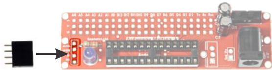
**Step 8 - Install the male header pins:** Break up the two male header strips each into a set of 22, 11, and 3 pins (as shown below). Solder the two sets of 22 and place them in the 'G' and 'V' locations (marked at the end of the PCB). The two sets of 11 are installed in the 'S' row, end-to-end.
