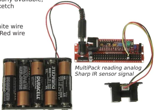
*MultiPack reading analog Sharp IR sensor signal*
