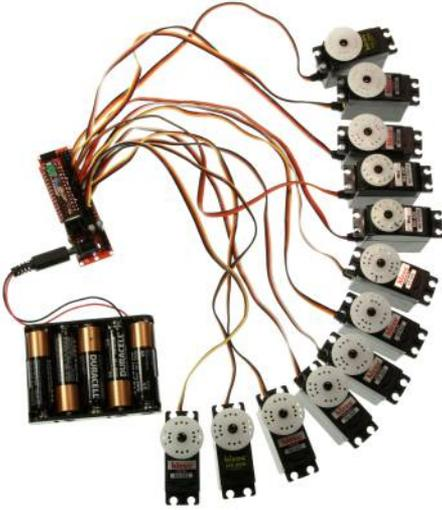
Our standard servo test using ports D2-D13 uses the default Arduino “Servo -> Sweep” Sketch, with the servos hooked up with:
