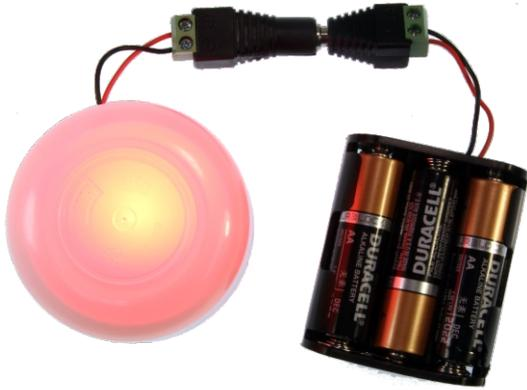
Select your favorite display mode, and cap it shut. The SB-Firefly remembers this setting, so will restart with it every time you plug in the battery pack, which will run the bundle for approximately 3 days on a fresh set of quality alkaline cells.
