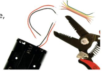
**Step 3 - Firefly Ribbon Cable:** Take a close look at your ribbon cable. Three of the wires will send the color signals, and the other two send the power. To keep wiring identification simpler, let's try to identify a side being "Power". Find one side of the cable with either a **red** wire or the **darkest** wire color, so we can use red to identify '+', or the darkest wire to identify '-'.
