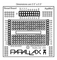
All I/O pins, Vdd, Vin, and Vss are routed through the AppMod connector.
