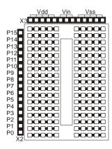
For chips with many legs (ICs), place them in the middle of the board so that half of the legs are on the left side and half are on the right side. Nodes on the left side are not connected to nodes on the right side.
